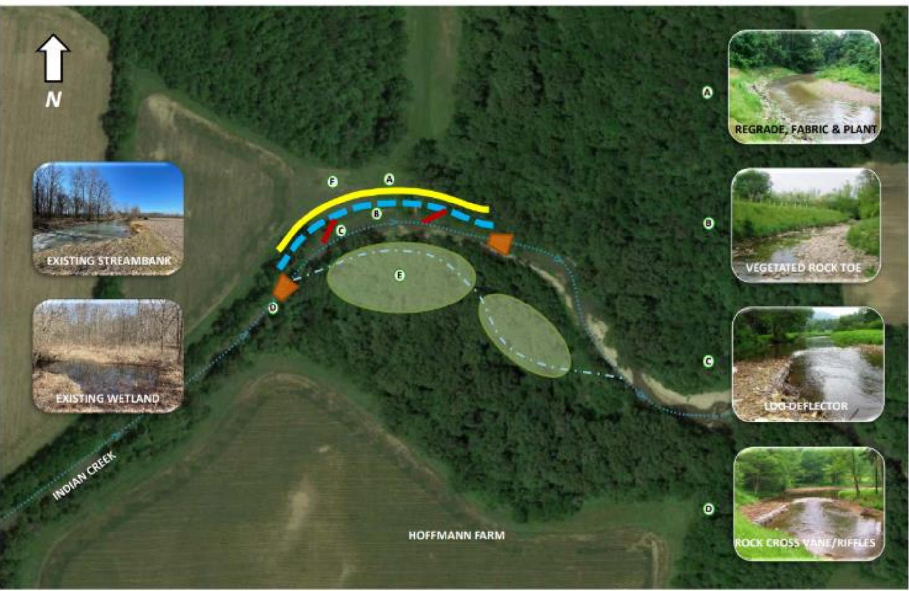
Figure 2. Conceptual Plan INDIAN CREEK - HOFFMANN WETLAND AND STREAM RESTORATION Approximate Scale: 1 in = 300 feet PLAN LEGEND* RIPIARIAN BUFFER ENHANCEMENT REGRADE, FABRIC & PLANT VEGETATED ROCK TOE PROPOSED FLOWLINE IMPROVEMENT ROCK CROSS VANE/RIFFLES LOG DEFLECTOR WETLAND ENHANCEMENT * Approximate locations
